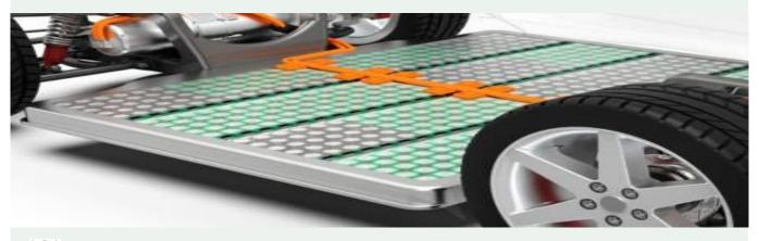
Efficient thermal management should maintain the proper temperature range and prevent high temperature gradients during the charge and discharge.
