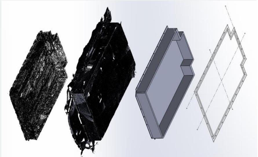
Figure 2. Battery tray and cavity validation
