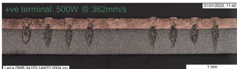
Figure 1. Welding parameters developed on empty cells for busbar-positive terminal and busbar-negative terminal joints.
