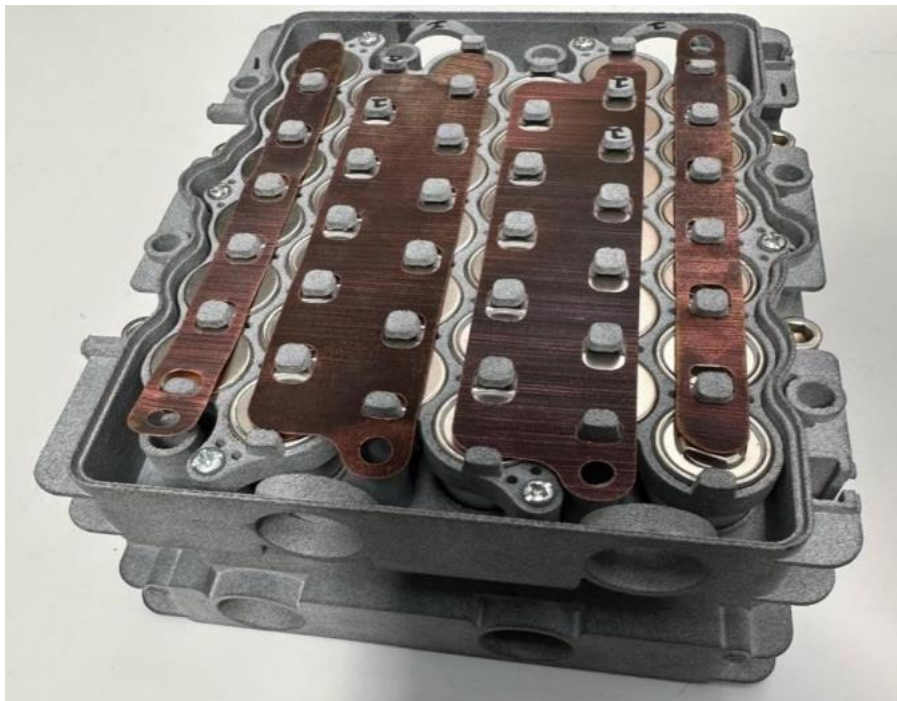
Figure 3. A dummy 6s6p 'mini-module', comprising 3D printed plastic cell holders (from the partner Cleantron), discharged cells (also supplied via Cleantron) and, in the example shown, DLIP textured Cu busbars (from the partner Fraunhofer IWS).
