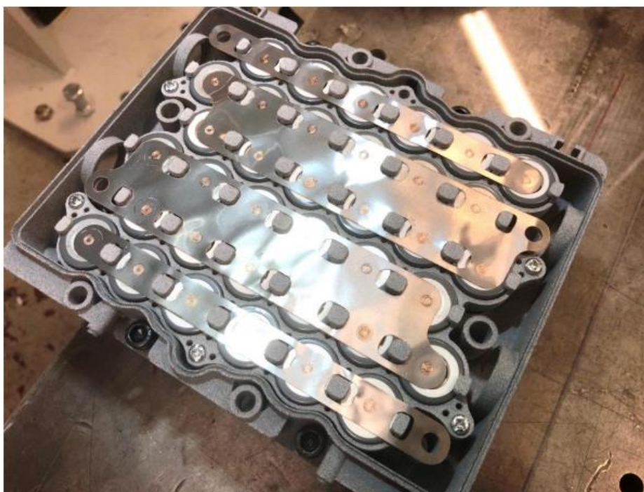
Figure 4. Examples of module welds into the positive and negative terminals of the dummy cells supplied by Cleantron.
