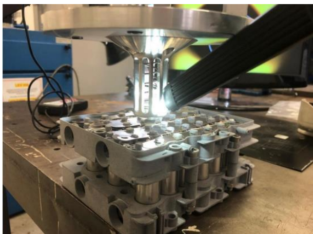
Figure 3. Clamping tool designed by TWI.
