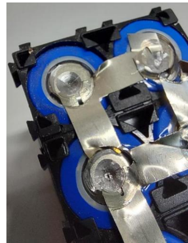
Figure 4. Setup for the dummy cells tests (left) and the respective dummy cells after employing the milling operation with a drill bit and the position control approach (right).
